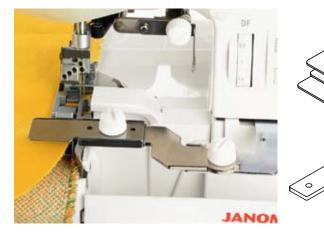
Attached to the machine, it guides curved fabric to straight edged, and is ideal for making table linens and bags with curves.
