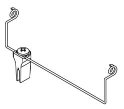
Prefer using industrial cone thread? Place unusually large thread cones behind the machine on the table and attach the guide to the antenna for smooth feeding of thread.
