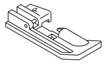
Beaded trims add that special touch to any project. Deep grooves on the bottom of the pearl foot guide strands of pearls or beads perfectly into place and are secured with a flatlock stitch.
