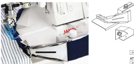
The tape binder clips on to the front of the machine and guides and folds 40 mm bias tape perfectly, doing away the need to pre-iron. Ideal for sewing straight fabrics to curved, finish difficult t-shirt necklines, etc with ease.
