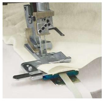
The elastic gathering foot not only takes the hard work out of attaching elastic, it is also great for making your own custom soutache. The three attachments allow you to sew 7.5 mm, 10 mm, or 13 mm flat elastic directly onto fabric. Adjust the screw to control the amount of tension or pressure placed on the elastic being gathered.
