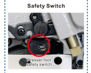
Presser foot safety switch provides protection in the whole process.
